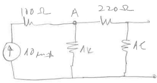
$$(V_A)_1 = 10 \text{ mA} \times \left( 1 \text{ k} \parallel (220 \Omega + 1 \text{ k}) \right)$$
