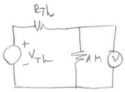
$V_{Mei} = \frac{1M}{1M + R_{Th}} \times V_{Th} = 5V$
