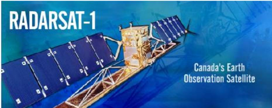
Launched in November 1995, **RADARSAT-1** provides Canada and the world with an operational radar satellite system capable of timely delivery of large amounts of data. Equipped with a powerful synthetic aperture radar (SAR) instrument, it acquires images of the Earth day or night, in all weather and through cloud cover, smoke and haze.
