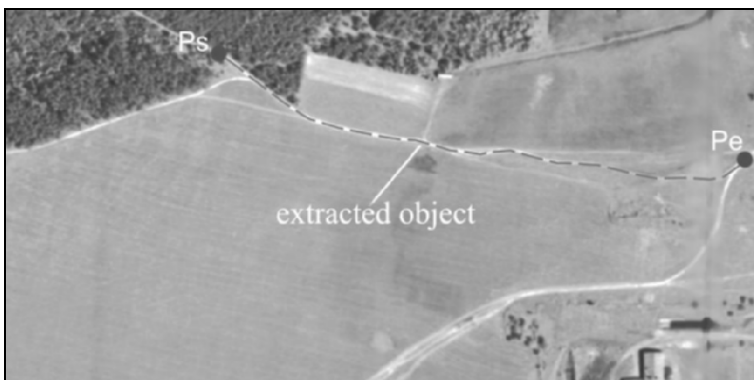
Figure 10. Result of road extraction (Ps: seed point. Pe: free point)
