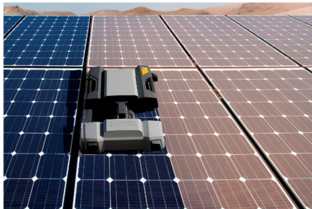
Figura 5: Robot de limpeza de módulos solares da Ecovacs Robotics. Fonte: https://www.solarpowerworldonline.com/2015/02/fighting-dirty-manual-washing-vs-automatic-cleaning-of-solar-modules/
