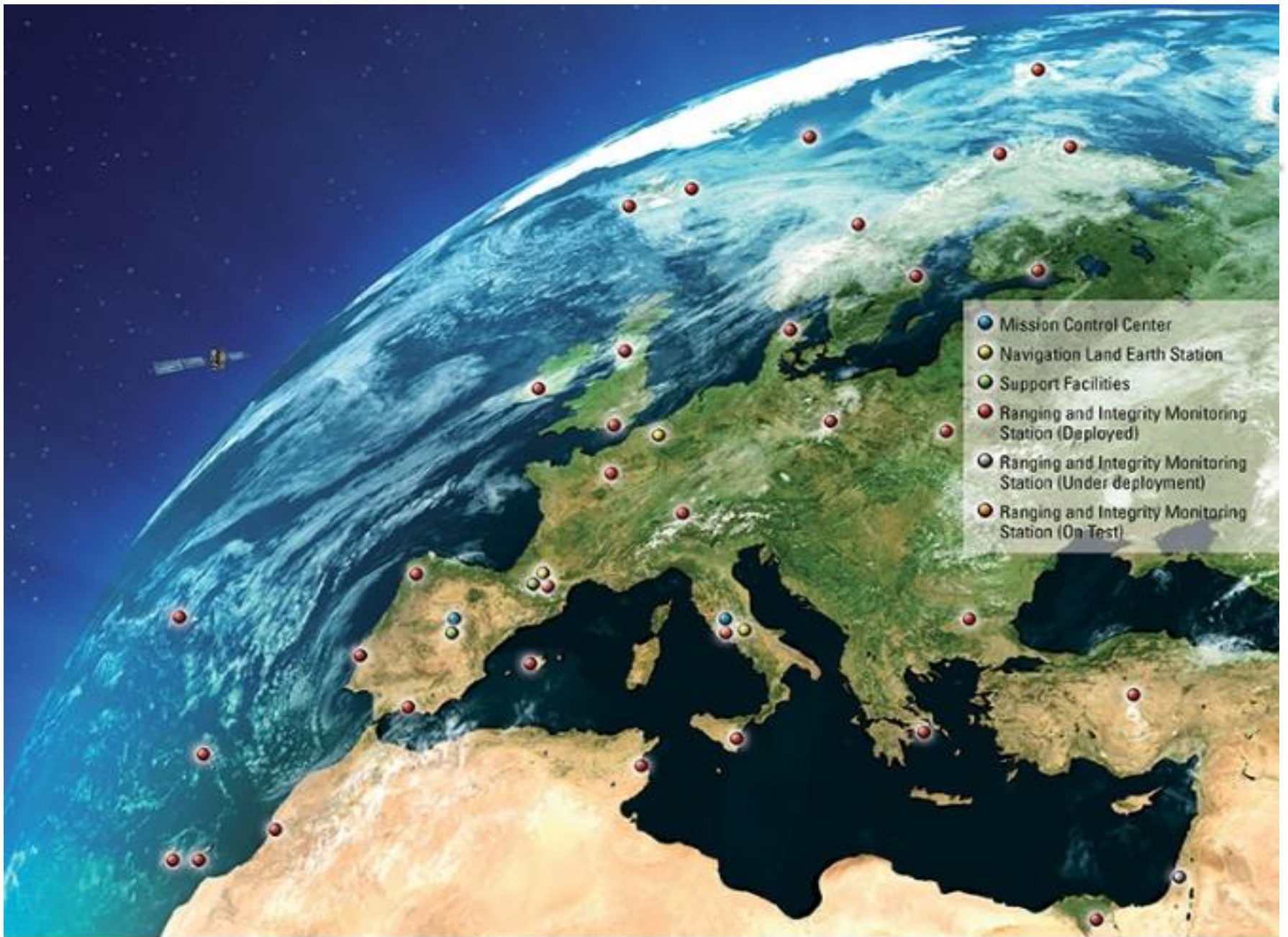
EGNOS ground segment, with locations of Support Facilities, MCCs, RIMs and NLES.
