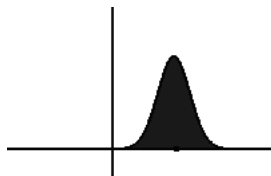
A solution to the one-dimensional Fokker-Planck equation, with both the drift and the diffusion term. In this case the initial condition is a Dirac delta function centered away from zero velocity. Over time the distribution widens due to random impulses.
