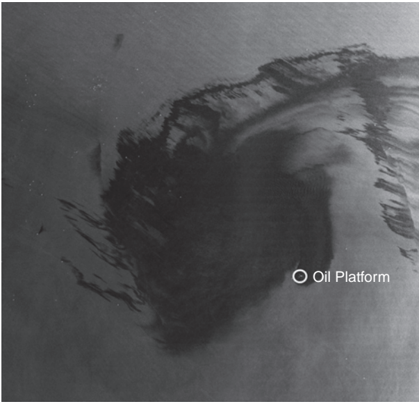
FIGURE 7. Oil pollution over the Gulf of Mexico acquired on April 30, 2010 (just 10 days after the explosion of “Deepwater Horizon,” leading to the largest offshore oil spill in U.S. history). Oil spills appear as dark areas in radar images because of the attenuation of the capillary waves, leading to a smoother ocean surface and decrease of the backscattered signal. Capillary waves are wind-caused ripple-waves with a wavelength less than a few centimeters. Image size: ca. 100 km × 100 km, acquired by TerraSAR-X in ScanSAR mode.
