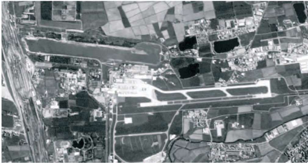
Figure 1-7: Optical image of Linate Airport taken from the SPOT satellite. No speckle is visible and the fields that surround the airport look homogeneous.
