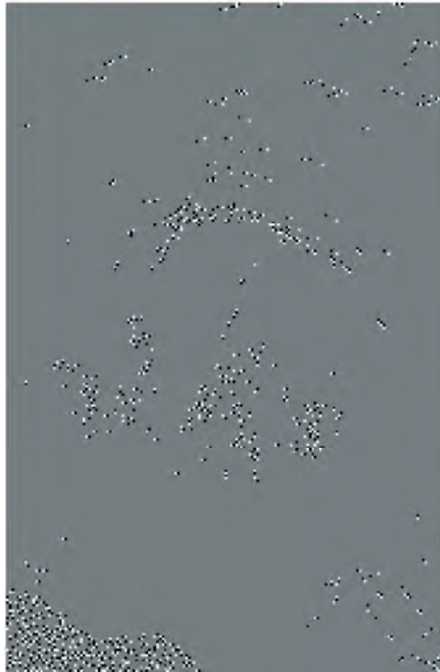
Figure 3-4: Map of the phase residues relative to the interferogram shown in Figure 3-2
