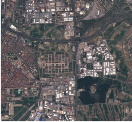
Figure 4: This image shows a Sentinel-2 satellite image in the RGB color space generated by combining the red (B04), green (B03) and blue (B02) spectral band. The shown image gives an impression of the visible objects at a spatial resolution of 10 meters per pixel.
