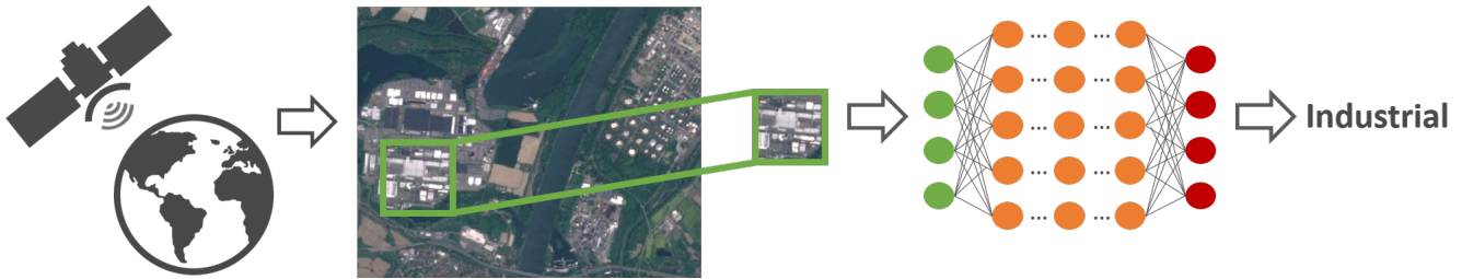
Figure 2: This illustration shows an overview of the patch-based land use and land cover classification process using satellite images. A satellite scans the Earth to acquire images of it. Patches extracted out of these images are used for land use and land cover classification. The aim is to automatically provide labels describing the represented physical land type or how land is used. For this purpose, an image patch is feed into a classifier, in this case a neural network, and the classifier delivers the land use or land cover class represented on the image patch.
