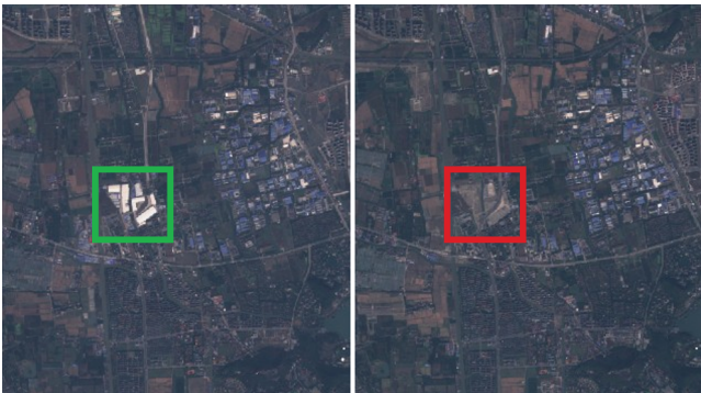
Figure 10: Change detection application 1a: The left image was acquired in the surroundings of Shanghai in December 2015 showing an area classified as industrial. The right image was acquired in December 2016 showing that the industrial buildings have been demolished.
