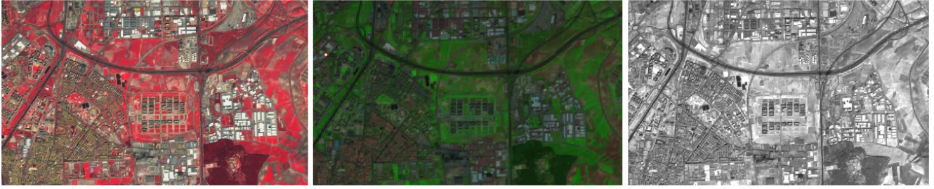
Figure 3: These images visualize different band combinations of the spectral bands provided by ESA’s satellite Sentinel-2A. The left image shows a color-infrared image by combining the near-infrared (B08), red (B04) and green (B03) band. The middle image displays a combination of the shortwave-infrared 2 (B12), red edge 4 (B08A) and red band (B04). The right image is constructed using merely the near-infrared (B08) band.
