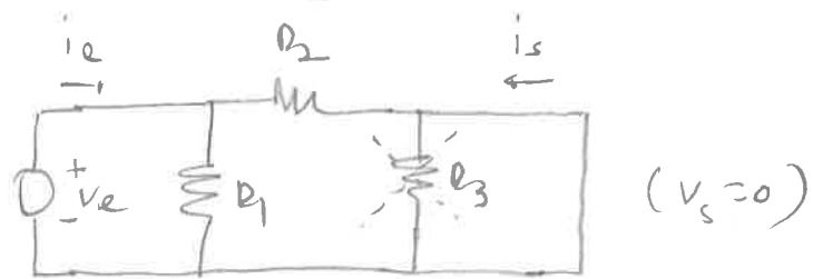
$$h_{11} = R_1 \parallel R_2 = \frac{R_1 \times R_2}{R_1 + R_2} = \frac{470 \times 220}{(470 + 220)} \approx 150 \Omega$$
