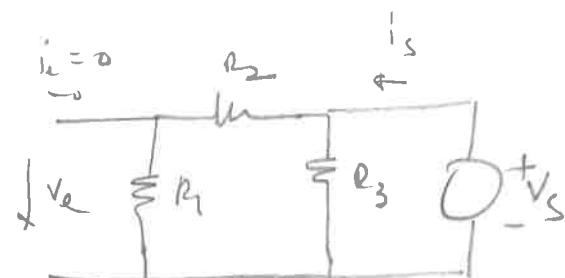
$$v_e = \frac{R_1}{R_1 + R_2} v_s \quad \Rightarrow \quad h_{12} = \frac{R_1}{(R_1 + R_2)} = 0,68$$
