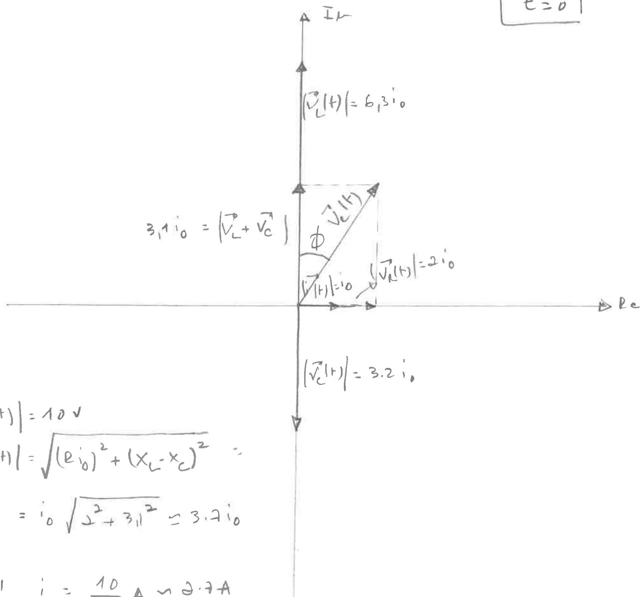
$$\begin{aligned} |\vec{V}_e(0)| &= 10 \text{ V} \\ |\vec{V}_e(0)| &= \sqrt{(E_i)^2 + (X_L - X_C)^2} \\ &= i_0 \sqrt{2^2 + 3,1^2} \approx 3,7 i_0 \end{aligned}$$
