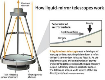
A liquid-mirror telescope uses a thin layer of
