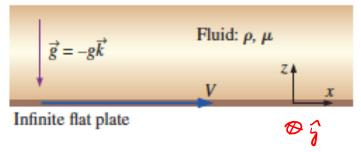
Consider a Newtonian fluid on top of a flat plate in the xy-plane at z = 0. The fluid is at rest until t = 0, when the plate suddenly starts moving at speed V in the x-direction.
