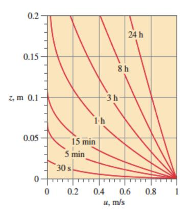
After 15 min of flow, the effect of the moving plate is not felt beyond about 10 cm above the plate!
