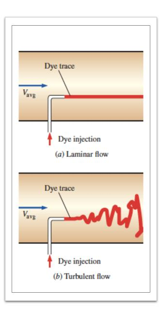
The flow regime in the first case is said to be laminar, characterized by smooth streamlines and highly ordered motion, and turbulent in the second case, where it is characterized by velocity fluctuations and highly disordered motion.
