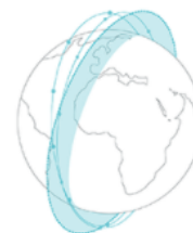
Planet's constellation of satellites orbit the poles every 90 minutes, capturing the entire Earth's landmass every day.
