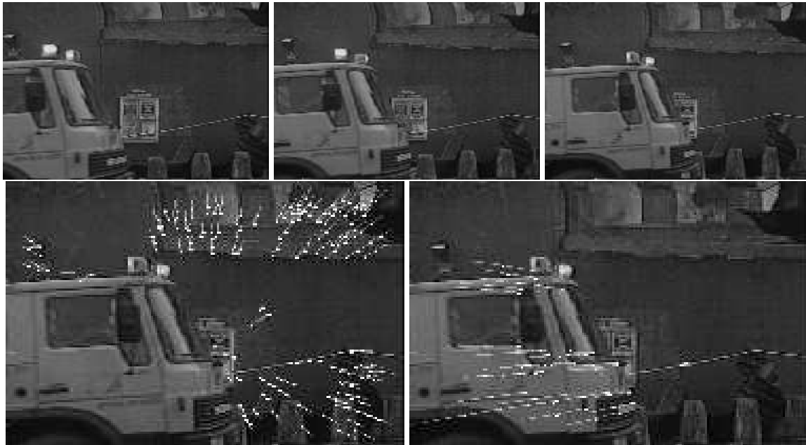
Figure 14: Three images of a sequence: the lorry move to the right, the camera moves away from the scene in a backward direction. The two images at the bottom show the two motions that were segmented: background and lorry. Images taken from: P. Torr, “Motion Segmentation and Outlier Detection”, PhD thesis, Oxford University, 1995.
