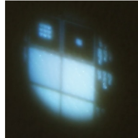
Figure 57 Photo of the Image on the Screen Created by the Keplerian Telescope Formed by the Field Lens and the Condenser Lens
