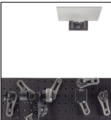
Figure 53: Positioning of the Beamsplitter Cube, Projection Lens, and Viewing Screen
