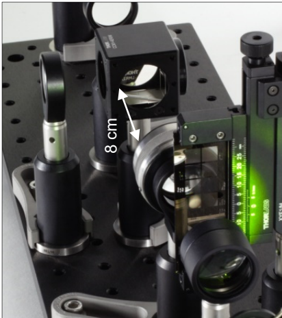
Figure 50: The holder of the beam splitter cube should not be illuminated.
