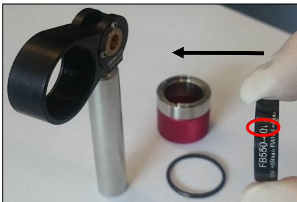
Figure 22: Assembly of the green filter: note the orientation indicated by the white arrow on the filter's mount.
