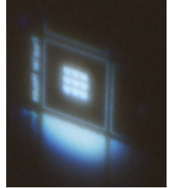
Figure 59: Photo of the Image on the Screen Created by the Keplerian Telescope Formed by the Condenser Lens and the Objective Lens
