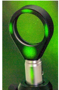
Figure 88 The first diffraction order does not fall on the lens.
