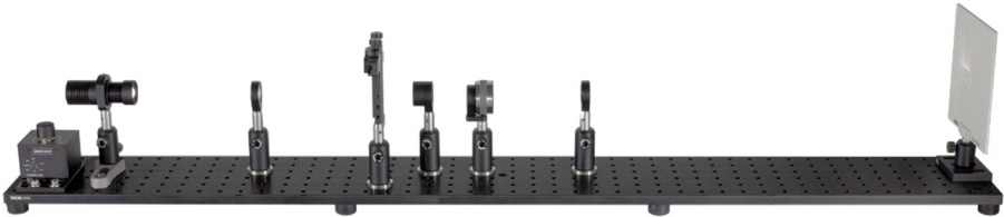
Figure 62: A lens projects the image from Exercise 2 onto a screen. In the Fourier Setup, this corresponds to the Fourier plane that is projected onto the screen (via the beamsplitter) since the camera-side focal plane of the objective lens is the Fourier plane.
