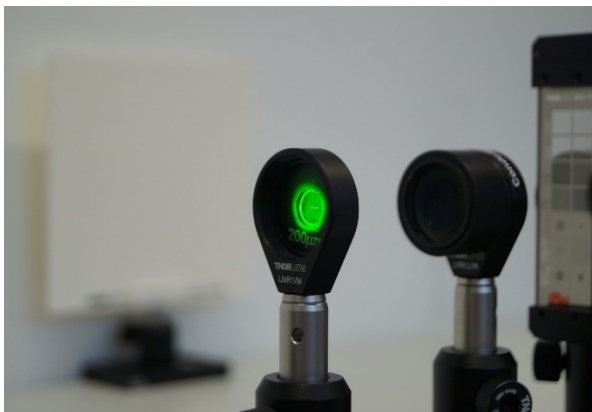
Figure 91: S200RD replaces the aperture iris in front of the condenser lens.
