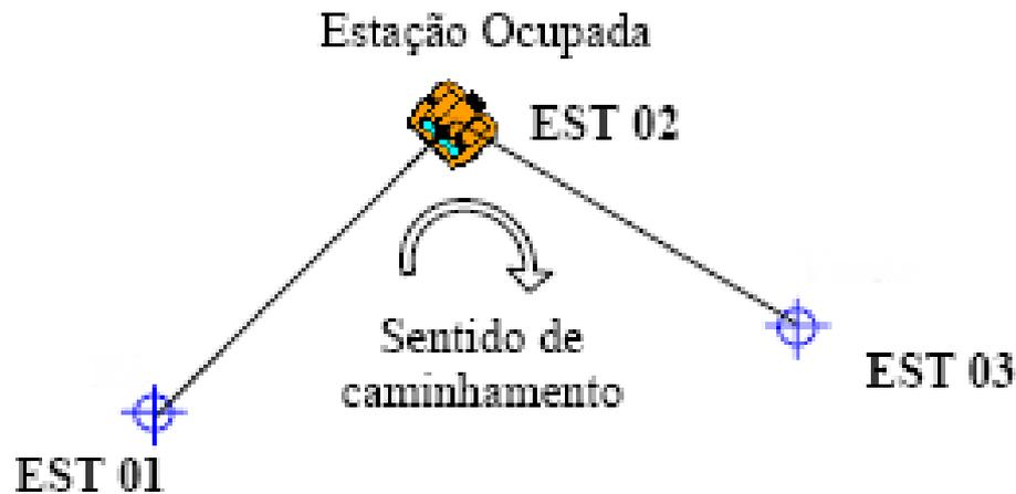
$$\text{Ângulo horizontal} = 287^{\circ} 39' 40'' - 15^{\circ} 02' 30'' = 272^{\circ} 37' 10''$$
