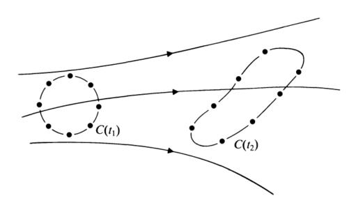
The inviscid equations of motion enter the proof only in helping to evaluate a line integral round C, so if viscous forces happened to be important elsewhere in the flow, i.e. off the curve C, this would not affect the conclusion that  $\Gamma$  remains constant round C.
