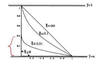
This flow resembles that of the unbounded plate until the boundary layer grows to the width of the channel. The solution then approaches the steady state  $u_s$ . Note that the slowest decaying exponential in the sum corresponds to n = 1. As a result, the flow reaches  $u_s$  on a time of order  $h^2/(\nu \pi^2)$ . For water in a 1cm channel, this time is about 10s and scales inversely with  $\nu$  so that in a fluid of lower viscosity it becomes longer.
