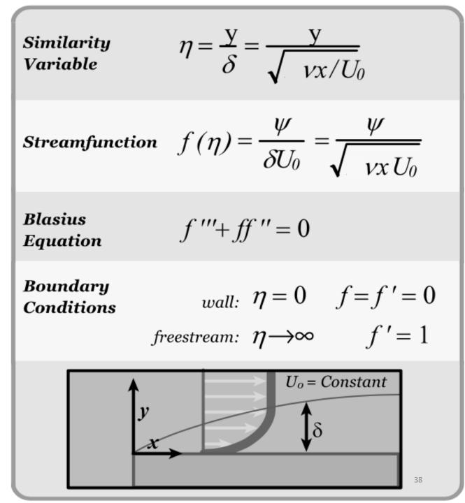
• Discussion: The Blasius boundary layer solution is valid only for flow over a flat plate perfectly aligned with the flow.
