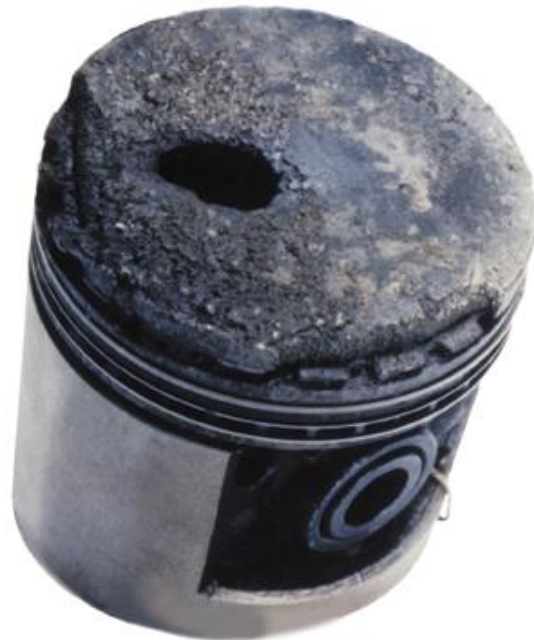
This photo of a badly damaged piston indicates the effects of long-term engine knock.
