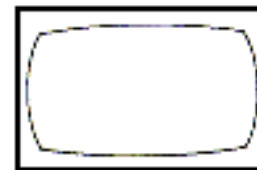
(g) Distortion due to Earth curvature
