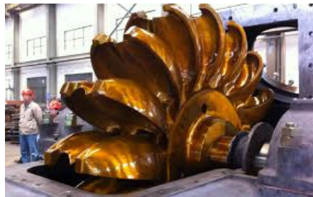
Pelton turbine (impulse turbine, high head, with vertical or horizontal shaft)
