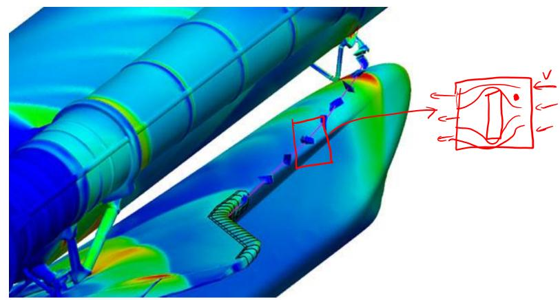
Forensic analysis of Columbia accident: simulation of shuttle debris trajectory using Eulerian CFD for flow field and Lagrangian method for the debris.
