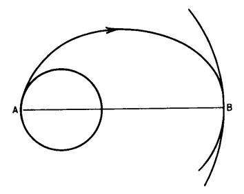
radius of the earth. This gives  $v^3 = 2\pi g R_0^2/\tau$ . Since the satellite is in a geostationary orbit,  $\tau = 24$  hours. This gives  $v = 3080 \text{ m s}^{-1}$ , and hence  $\delta v = 34 \text{ m s}^{-1}$ .
