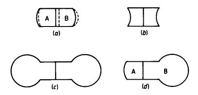
equilibrium if E is a minimum, i.e. if  $\partial^2 E/\partial R^2$  is positive. The expression for  $\partial^2 E/\partial R^2$  is of the form  $aR + b + c/R^3$ , where all the coefficients are combinations of physical magnitudes already defined, and must be positive. Thus  $\partial^2 E/\partial R^2$  is positive for all positive values of R, and the equilibrium, wherever it may be, is stable.
