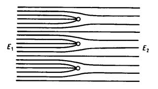
drop along one mean free path is large enough. If the drift is from  $E_1$  to  $E_2$  this would have the effect of increasing the apparent fraction reaching the  $E_2$  region. If the wires are very fine, then the high local field near their surface may give rise to field emission, independent of the impact of electrons.
