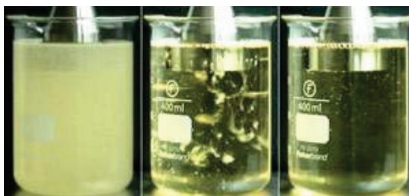
Figure 5.3: Degassing oil by applying ultrasonic vibration. The process takes about 5 seconds. (courtesy Hielscher Ultrasonics GmbH)
