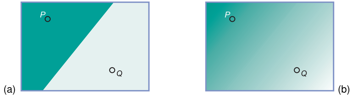
Figure 5.13: A geographic field representation obtained from two point measurements: (a) for qualitative (categorical), and (b) for quantitative (continuous) point measurements. The value measured at P is represented as dark green, that at Q as light green.
