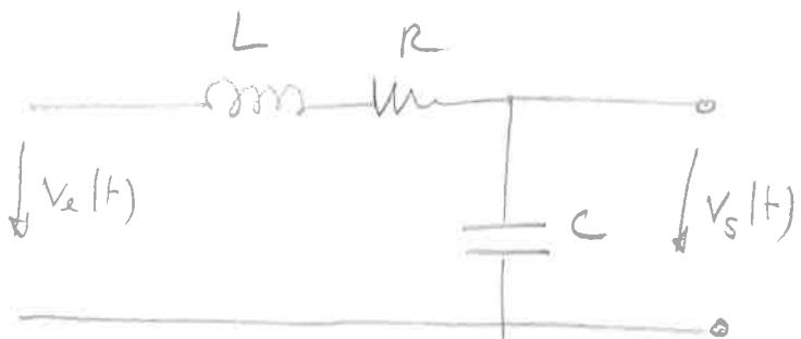
$$a) \vec{Z}_{\text{TOTAL}} = \vec{Z}_L + \vec{Z}_R + \vec{Z}_C = j\omega L + R + \frac{1}{j\omega C} =$$
