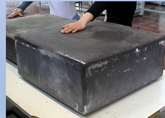
Typical casting: 240kg/56 hours
